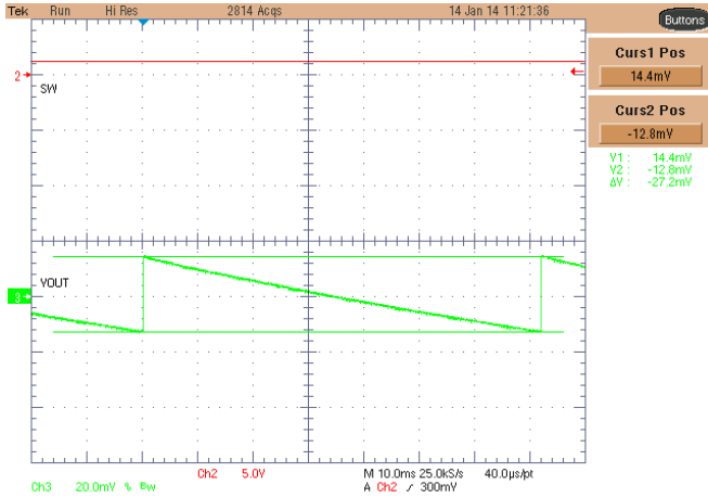
Figure 12. DCDC1 Ripple Voltage in PFM Mode ( V_{IN} = 3.6\text{ V} - V_{OUT} = 1.2\text{ V} - \text{No load} )
