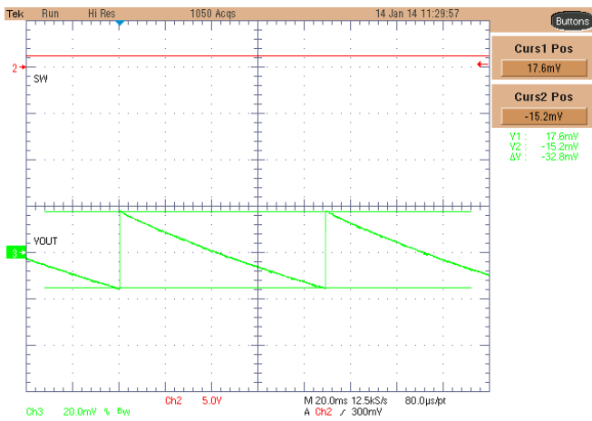
Figure 14. DCDC2 Ripple Voltage in PFM Mode ( V_{IN} = 3.6\text{ V} - V_{OUT} = 1.2\text{ V} - \text{No load} )
